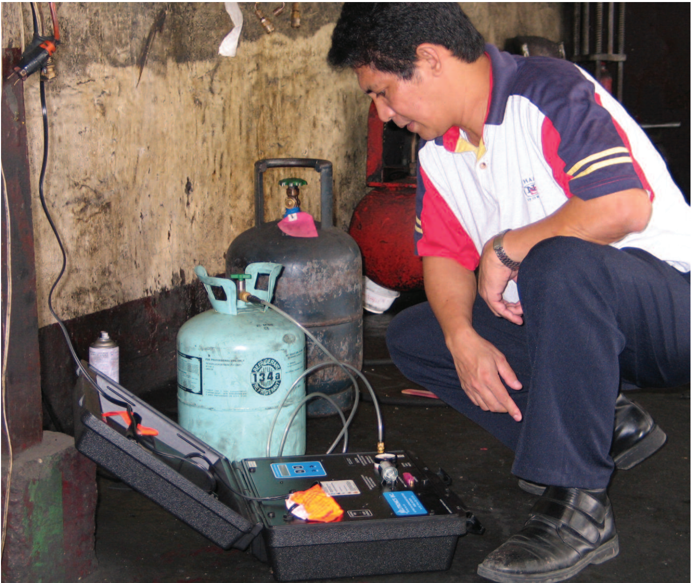
A government official in the Philippines tests counterfeit cylinders labelled as HFC-134a but containing CFC-12.
