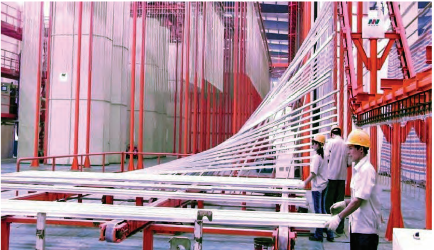
Vertical fluorocarbon painting system. HCFC-22 feedstock use for teflon and other polymer production has increased dramatically.
