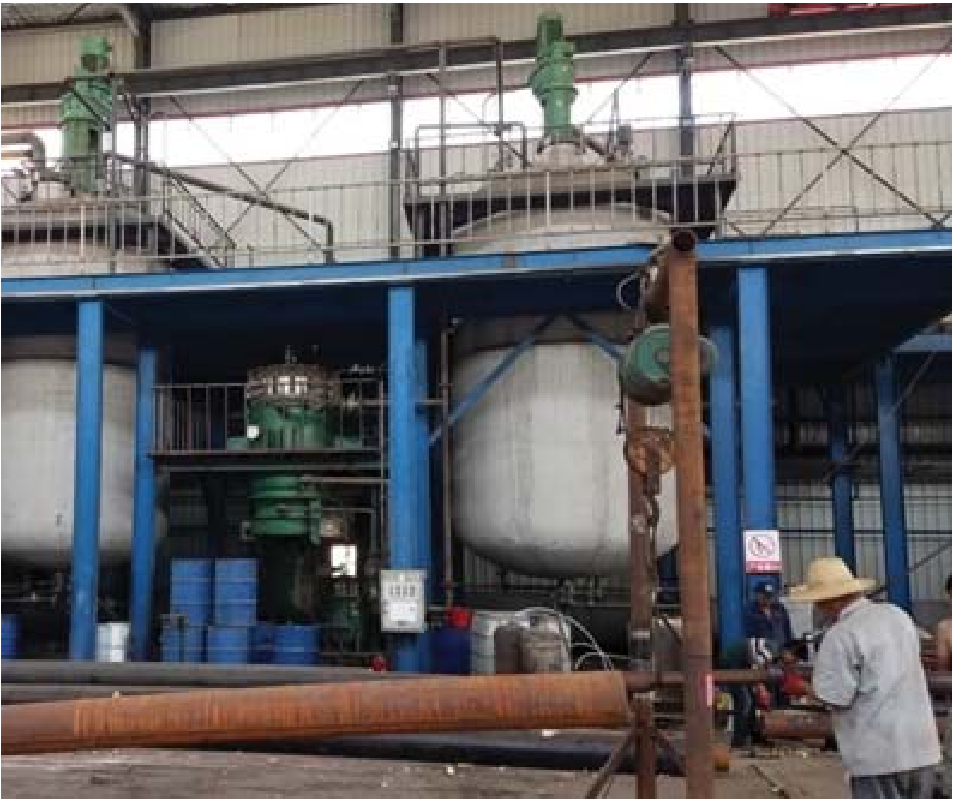
Image taken at Dacheng Aoyang Chemical Co.Ltd: two tanks with mixtures for white agent (polyol blend)
